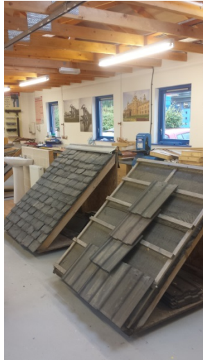
Picture 1 Structures for roof tiling. Peebles High school.
